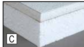
C. 1-1/2-inch EPS Foam is laminated to 1/2-inch fire and moisture-resistant gypsum and FiberLite FRP one side only. 2 feet x 4 feet.
