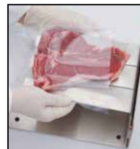
Fingers are removable and adjustable. Guide allows fingers to move easily from side to side.
