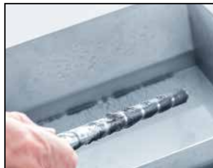
Magnetic bar collects dirty abrasion in water tray.
