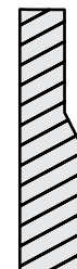
Cross section of Brute belly patch. Patch is cured directly into fabric.
