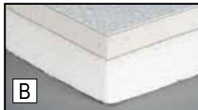
B. 1-inch EPS Foam is laminated to 1/2-inch fire and moisture-resistant gypsum and FiberLite FRP one side only. 2 feet x 4 feet.
