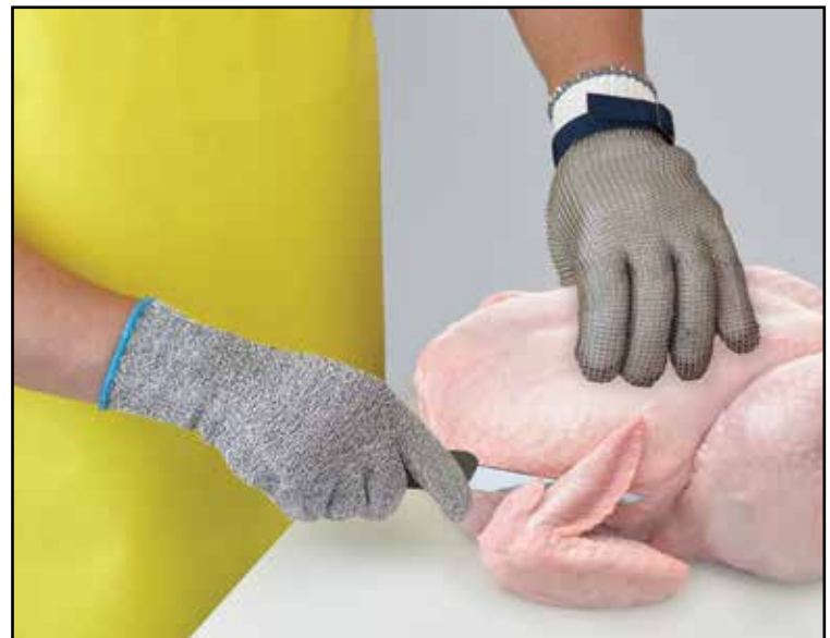
Cut-Resistant Glove can be worn on knife hand, when a metal mesh glove is used. Cut-Resistant Glove can be worn on non-knife hand, when a metal mesh glove is not used.
