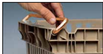
Two 3/8 inch zinc-plated steel wire bails swing down to allow nesting and swing up for stacking.
