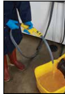
Remote high flow bucket/autoscrubber fill gun.
